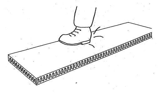
If you need to walk on the panels, the panels should be protected by using a 15 mm thick plywood board.
